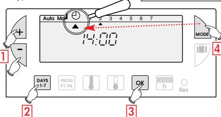
**1** Set the time using the **+/**- buttons (the numbers run off more quickly when the button is pressed continuously).
