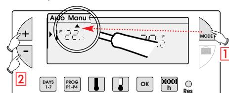
**1** Press the **MODE** button to position the pointer **▲** under **Manu**.
